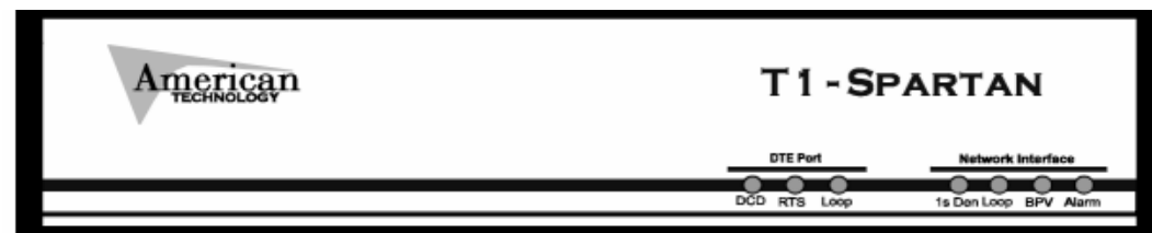
Figure 2-1. T1 Spartan T1/FT1 CSU/DSU Front Panel View
