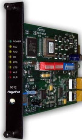
Figure 2-1. Front View of Modem
