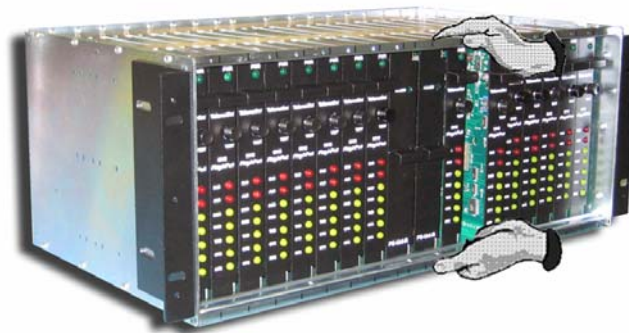
Figure 2-3. Installing the Modem
